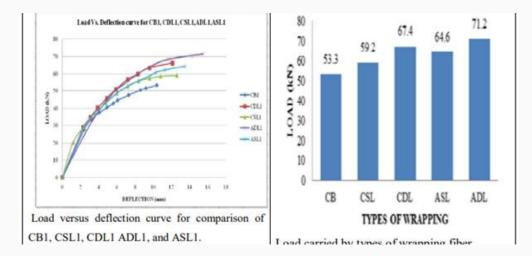
CB – Control beam, CSL – Carbon Single layer wrapping, CDL – Carbon Double layer wrapping, ASL – Aramid Single layer wrapping, ADL – Aramid Double layer wrapping.
