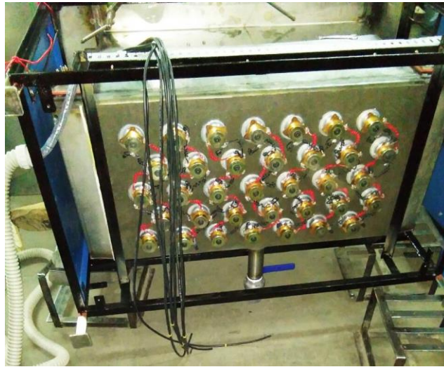
Photograph 5- Ultrasonic Cleaning System tank -Sensor arrangement at surface of tank
