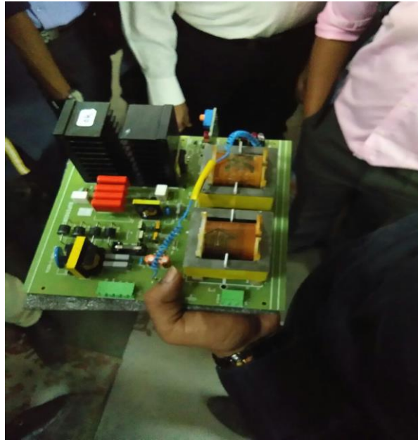
Photograph 3- Ultrasonic Cleaning System tank -Generator Circuit
