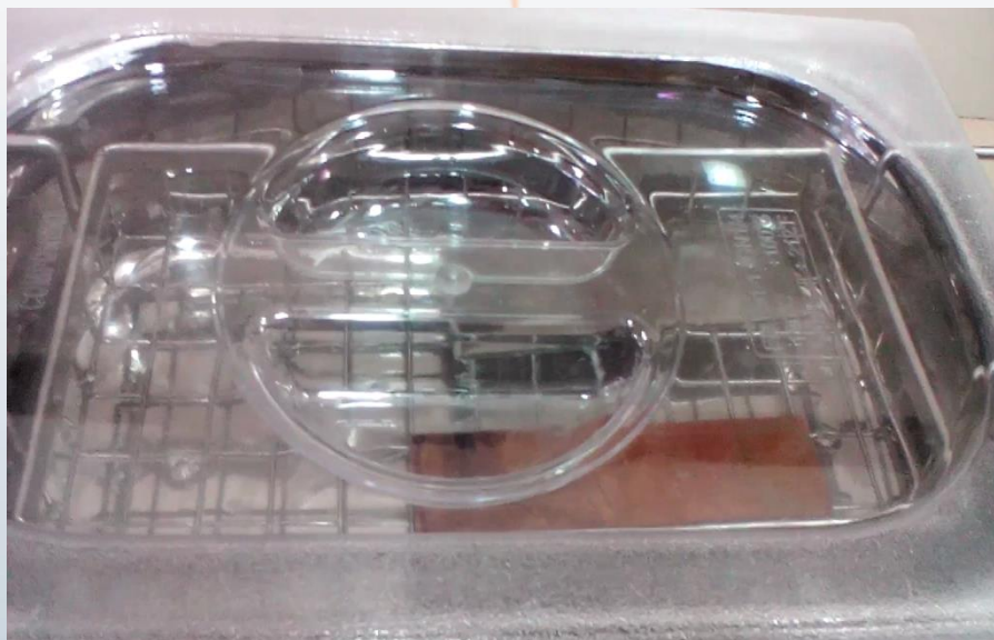
Photograph 4- Ultrasonic Cleaning System tank -Small bucket cleaner
