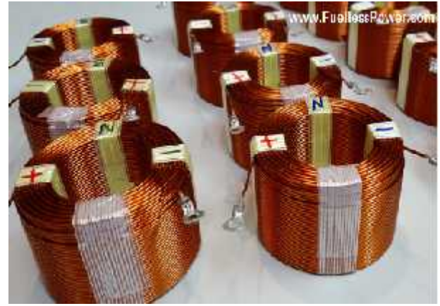
Fig. 5: Generator coils (Copper)
