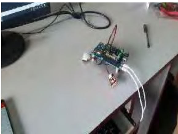
Fig.2 Arduino connected to Infrared motion sensor and Light sensor
