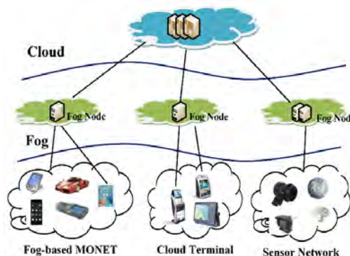
Fig 1. Architecture of Fog computing
