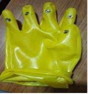
Fig4. Glove and the Metallic buttons
