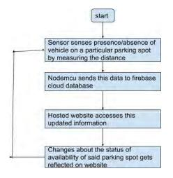
Fig 1: System Architecture (Flowchart)
