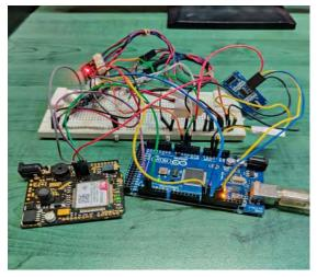
**Fig, VIII: The Hardware of the System** The internal connections of the hardware kit are demonstrated in the above figure which include Ardiuno MEGA, GSM module, Accelerometer etc.
