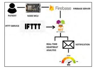
Figure No 6.2 Heart Rate Detection and Monitoring using Pulse Sensor Band.
