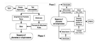
Figure 5: Phases of TTS synthesis process
