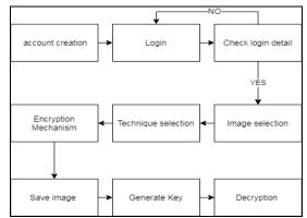
Fig: Flowchart for how our system works.
