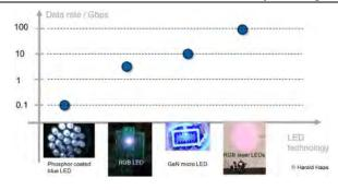
Fig.4.2 LED vs Data Rate
