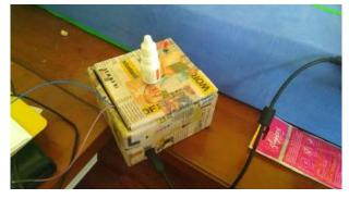
*Fig 4: Smart Medicine Box- System is active and waiting for the time of medicine to be taken. LED is turned off.*
