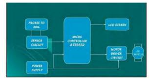
Fig: System Design Diagram for Smart Irrigation System 3.3 WORKING OF THE CIRCUIT
