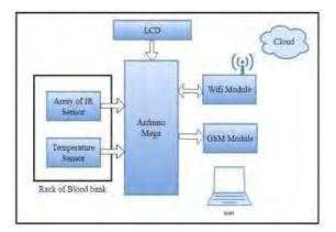
Figure -2: Block diagram of IoT Based blood bank system
