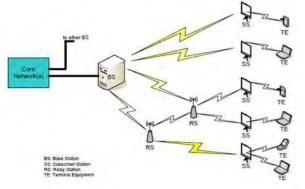
Figure 6: Wi-Max network architecture
