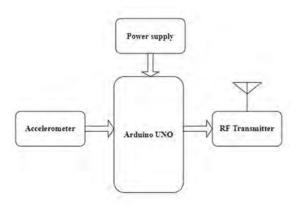
Figure A Block Diagram of Transmitter
