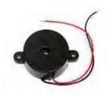
Fig.3.5 Piezo buzzer
