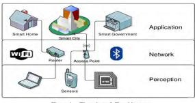
Figure 1. Three-layer IoT architecture.
