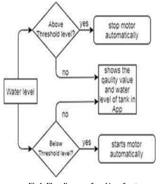
Fig 1: Flow diagram of working of system Features
