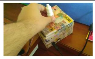
Fig 6: Smart Medicine Box- As the patient lifts the medicine for intake; the LED will glow continuously until medicine is kept back on place. The system will then again until the next time arrives VIII. RESULTS
