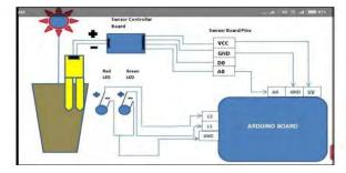
Fig: Working of the Circuit for Smart Irrigation System
