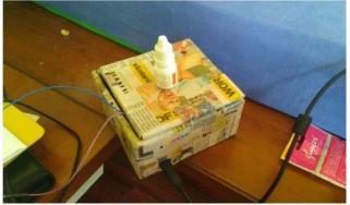
Fig 5: Smart Medicine Box- LED starts to blink when the time take the medicine was set and it will keep on blinking until the user picks up the medicine on the box.
