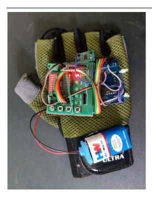
Figure C Prototype of Transmitter
