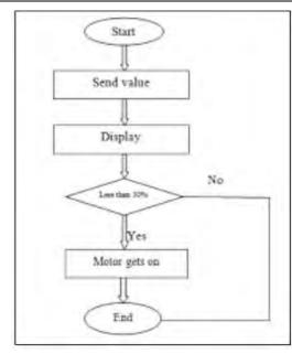
Fig: Flowchart for Smart Irrigation System
