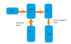
FIG 1X.1 block diagram of IoT based Child Tracking System.
