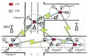
Fig. 1. Clustering of Vehicles in VANETs.
